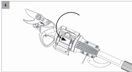
4. Close the tool attachment system (1) around the electric pruning shears (FELCO 802, FELCO 802G, FELCO 812 or FELCO 822).
