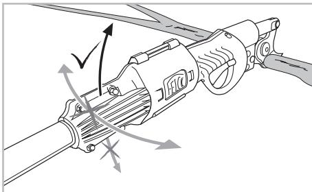
Disconnect the electric pruning shears and the cable connector from the extension poles connector while storing the FELCO 880/100-100 and/or FELCO 880/100-150 extension poles.
