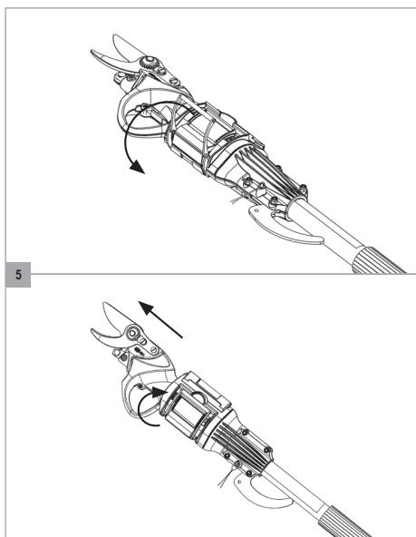
5. Close the attachment system by closing lever (8), which must be fixed to the opposite shell. Lock the attachment system by locking closely it against the shell. Make sure that the attachment system closing lever (8) is locked. No part of the attachment system closing lever (8) must be free to move when the extension poles are in use.
