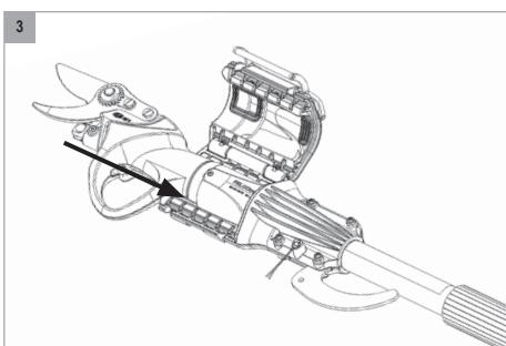
3. Insert the electric pruning shears (FELCO 802, FELCO 802G, FELCO 812 or FELCO 822) into the tool attachment system (1), making sure they are correctly positioned.
