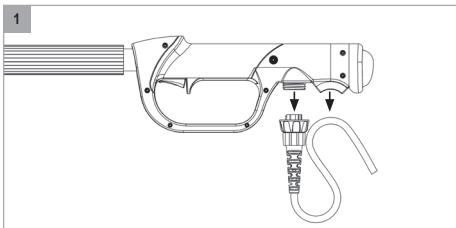
1. Make sure that the cable connector is disconnected from the FELCO 880/100-100 and/or FELCO 880/100-150 extension poles.
